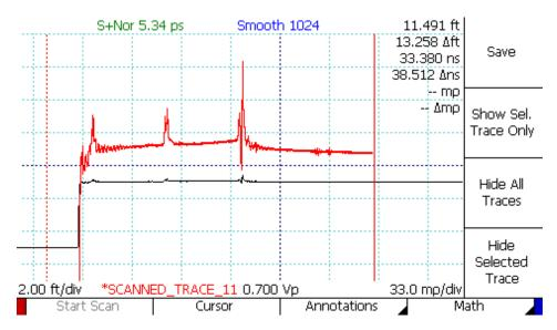
**Figure 4.18.** Scan of a portion of a cable (red), zoomed-in vertically to show additional detail relative to the live trace (black).
