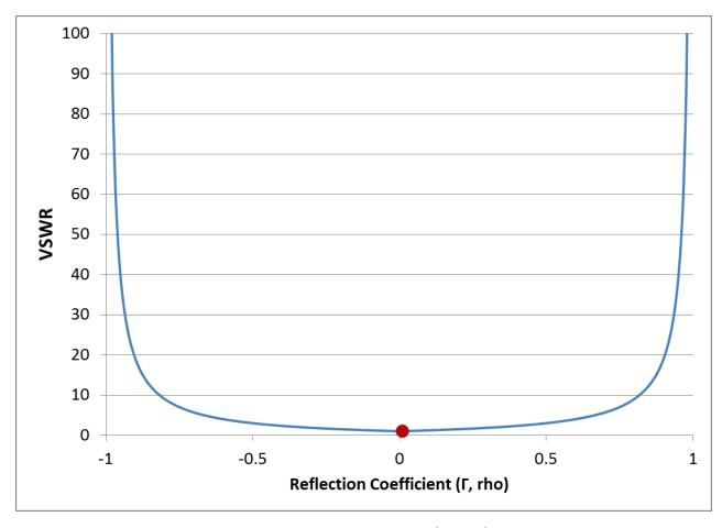
**Figure 7.8.** Relationship of voltage standing wave ratio (VSWR) to reflection coefficient (rho). VSWR for 50 ohm load is shown by the red circle.
