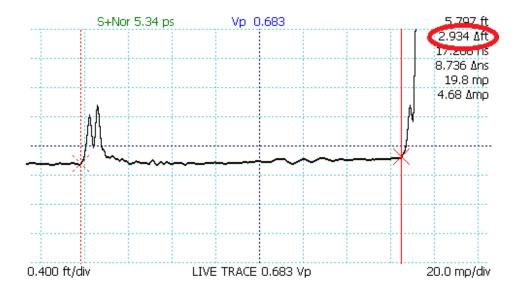
**Figure 4.12.** Relative distance measurement between two small impedance "faults" caused by BNC connectors.
