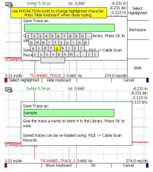
**Figure 4.30.** Using the on-screen keyboard. Choose Hide Keyboard when finished. Then choose OK to save the trace with the name you entered.
