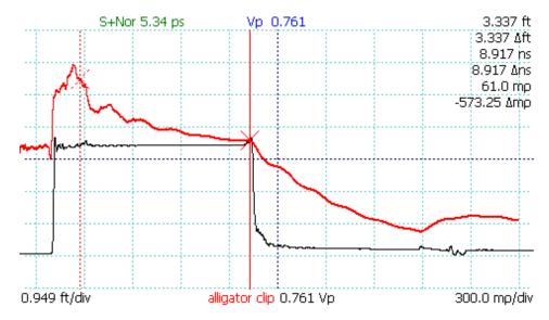
**Figure 4.1.** Clip lead adapter (red, top) and controlled-impedance adapter (black, bottom) testing of 3 ft. coaxial cable with short termination. Active cursor is at the test port. Clip lead adapters introduce severe TDR trace distortion.
