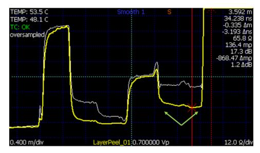
**Figure 5.10.** Example layer-peeling trace (yellow, bottom) versus live TDR trace (white, top). The layer peeled trace reduces the impedance error in the final cable segment (green arrows) by  $\sim 80\%$ .
