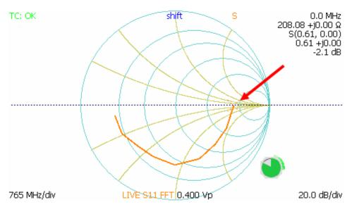
**Figure 5.14.** Smith chart of reactive 200 ohm load showing effect of reactive impedance at higher frequencies. Cursor (red arrow) shows impedance value calculated at DC (0 MHz).
