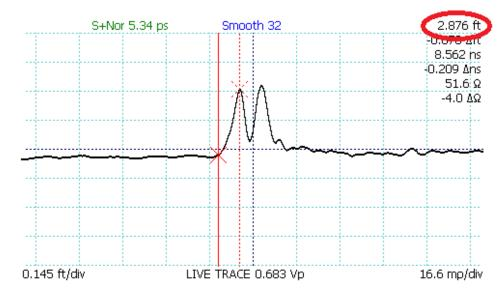
**Figure 4.11.** A horizontally zoomed-in view of the cable fault with active (solid) cursor at the start of the fault ("toe" region) and inactive (dashed) cursor at the peak of the fault. The DTF measurement is highlighted (red circle).
