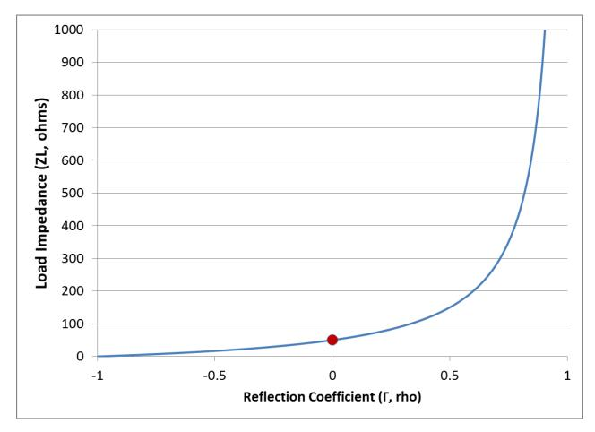
**Figure 7.6.** Relationship of impedance (ohms) to reflection coefficient (rho) for 50 ohm source impedance (marked by red circle).
