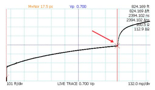
Figure 7.3. An open cable fault at 824 ft.
