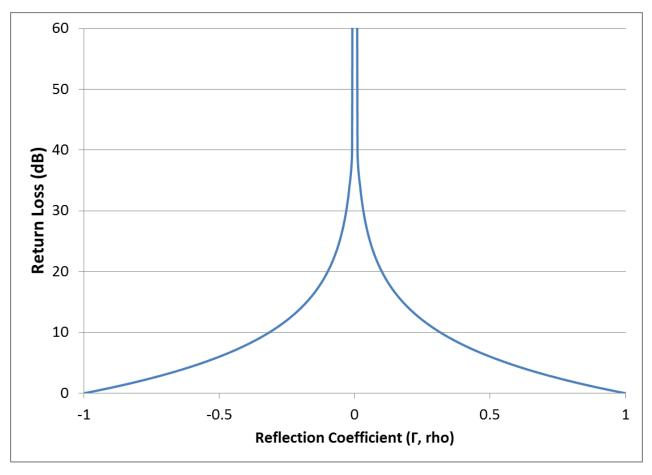
Figure 7.7. Relationship of return loss (dB) to reflection coefficient (rho).
