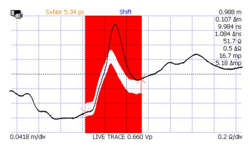
Figure 4.34. A trace that fails the mask test.
