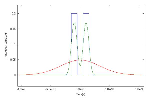
**Figure 7.9.** Simulated comparison of a 90 ps rise time TDR (green) and an 800 ps TDR (red) with respect to the ability to depict two 1 cm long, 75 ohm faults spaced 1 cm apart on a 50 ohm cable. Notice how the faster TDR (90 ps) resolves each fault individually. The blue lines represent a theoretically perfect response.
