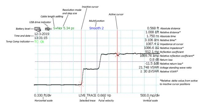
Figure 3.9. Screenshot showing typical features of the CT100B.
