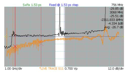
**Figure 5.7.**  $S_{11}$  between cursors with loosened connector showing average return loss of -26.7 dB from 756 MHz to 3 GHz (7.7 dB excess return loss compared with the tightened connector in Figure 5.6).
