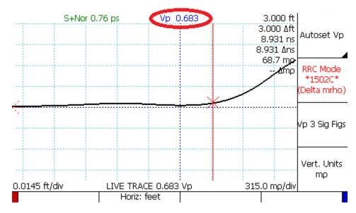
Figure 4.7. Final Vp of the cable.
