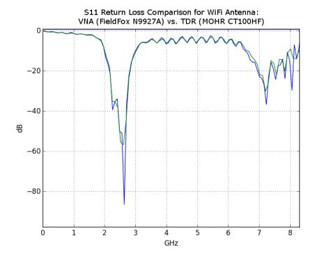
**Figure 7.10.** Comparison of  $S_{11}$  return loss of a 2.4 GHz WiFi patch antenna measured using a handheld VNA (Agilent® FieldFox N9927A, green) and TDR (CT100HF, blue), showing good agreement from DC to ~8.3 GHz. Note bandpass in the 2.4 GHz region.
