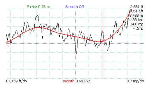
**Figure 4.8.** Smoothed vs. unsmoothed traces at very small vertical scales (0.7  $m\rho$  per vertical division).
