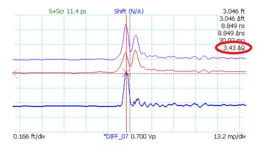
**Figure 5.1.** Difference trace. Live (base trace, purple, top), comparison scan (red, middle), difference (blue, bottom) traces show 3.43 ohm excess impedance (red circle) on the live trace due to a loosened BNC connector.
