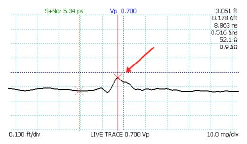
Figure 4.4. A scan of an SMA connector.
