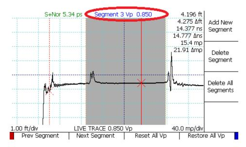
Figure 4.17. Multi-segment cable segment with Vp of 0.850 (red circle).
