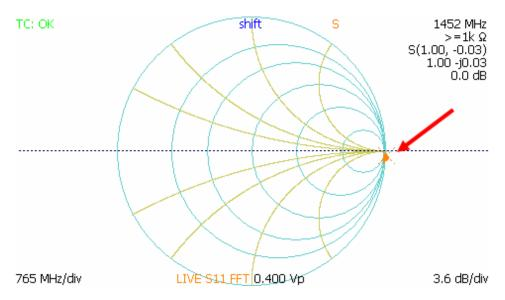
Figure 5.11. Smith chart representation of open fault (red arrow).
