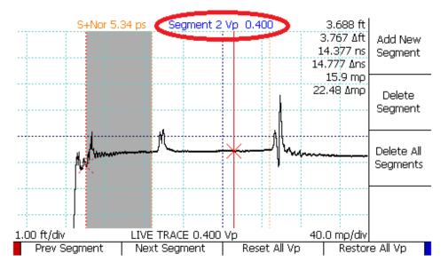
Figure 4.16. Multi-segment cable segment with Vp of 0.400 (red circle).
