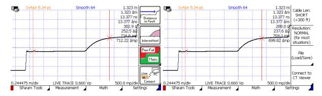
**Figure 3.6.** The two versions of the Main menu. On the left is the Special menu and on the right is the Standard menu. Note that the menu selections across the bottom are exactly the same for both menus.
