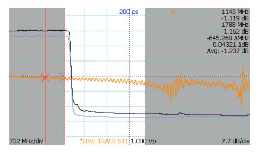
Figure 5.9. Normalized trace (blue, bottom) showing short fault in a 50 ohm cable.
