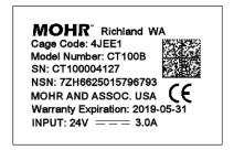
Figure 3.1. Example nameplate label found on back of a CT100B.
