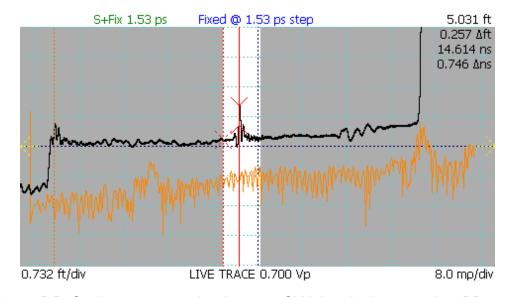
**Figure 5.5.** S<sub>11</sub> between cursors bracketing an SMA barrel adapter on the TDR trace.
