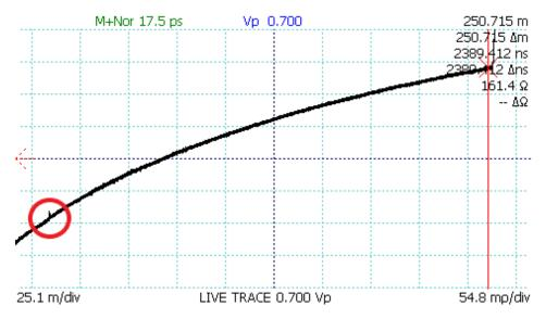
**Figure 3.10.** A small fault in a long cable. This fault (red circle) in an approximately 800 ft. (250 m) cable is from a 3 cm barrel connector (0.01% of cable length). The sampling of the Normal sample resolution setting ensures that the cable fault is displayed at this large horizontal scale ( $\sim$ 50 cm/pixel).
